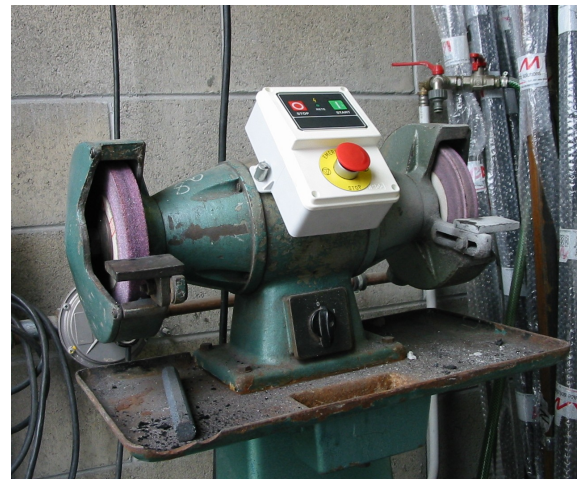
Electrical safety control panel for motors up to 10 hp
